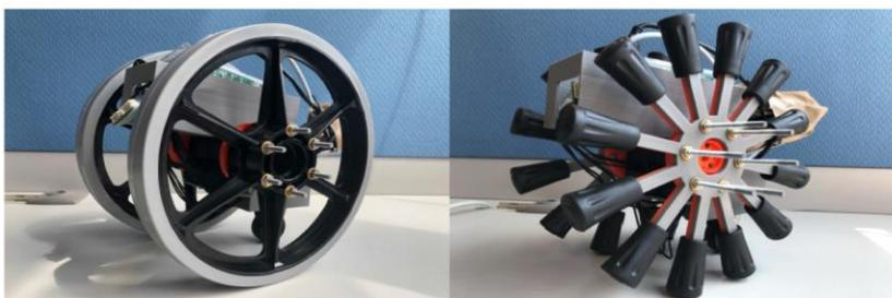
Wheel robot and rimless wheel robot
